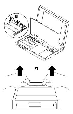
After replacing the diskette drive, latch the removal strap into the correct position.
